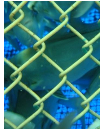
Figure 5: Copper Alloy after 4 weeks in the net pen
