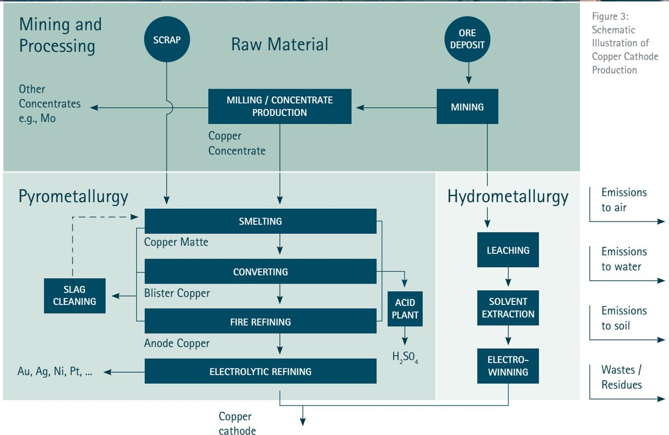
Figure 3: Schematic Illustration of Copper Cathode Production
